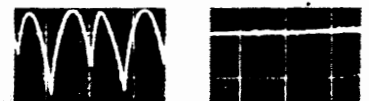
Actual oscillograph traces illustrate dramatic improvement of suction pressure conditions with Suction Stabilizer.
